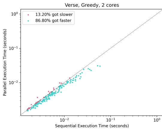
Figure 14: The speedups acquired with two cores using the greedy algorithm, for the verse benchmark. It can be observed that the number of candidates that achieved a speedup increased, compared to using the deterministic algorithm.
